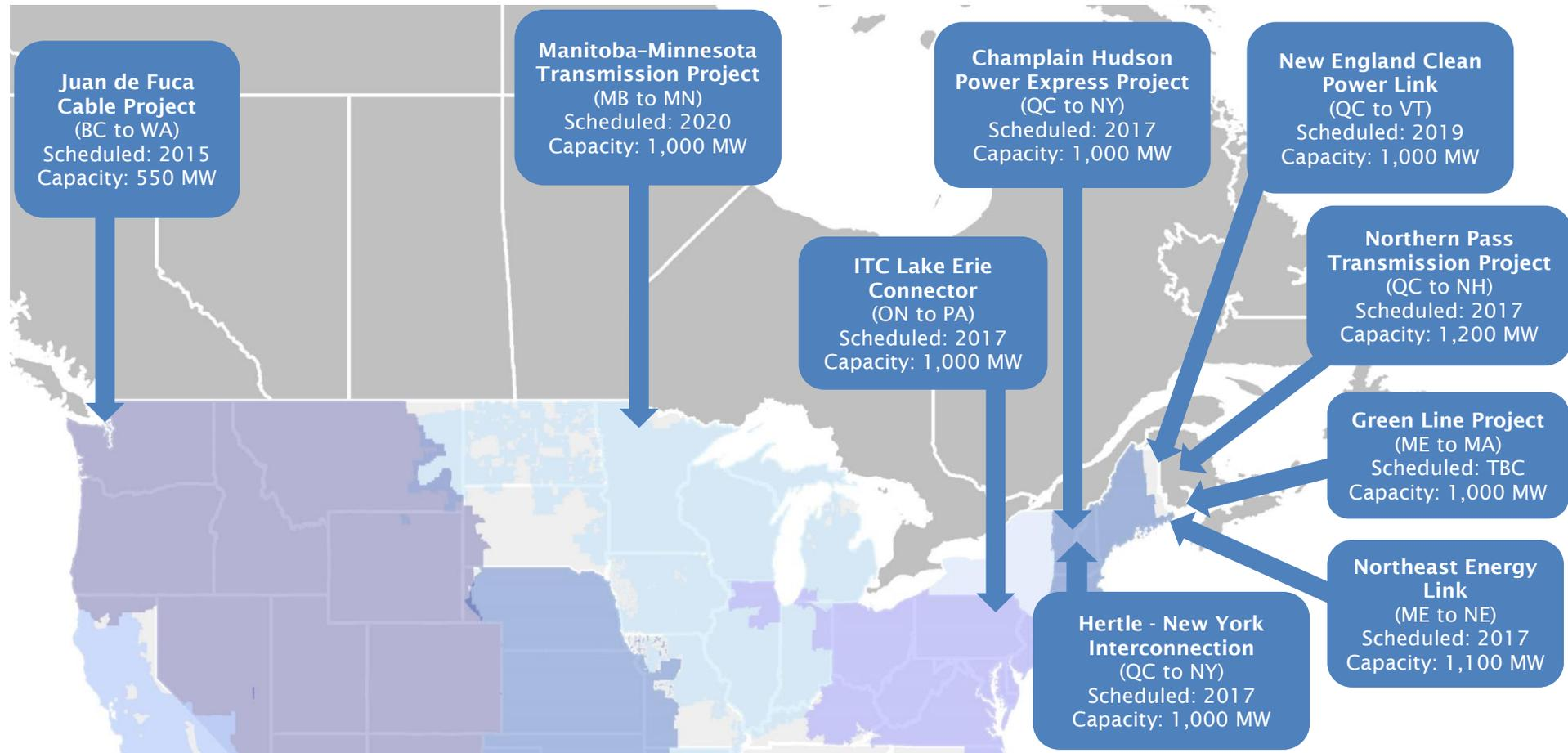
Almost 80% of proposed cross border transmission capacity is focused on Eastern US markets, because of the current appetite for large scale low carbon/renewable resources to diversify the predominantly gas-fired supply mix
